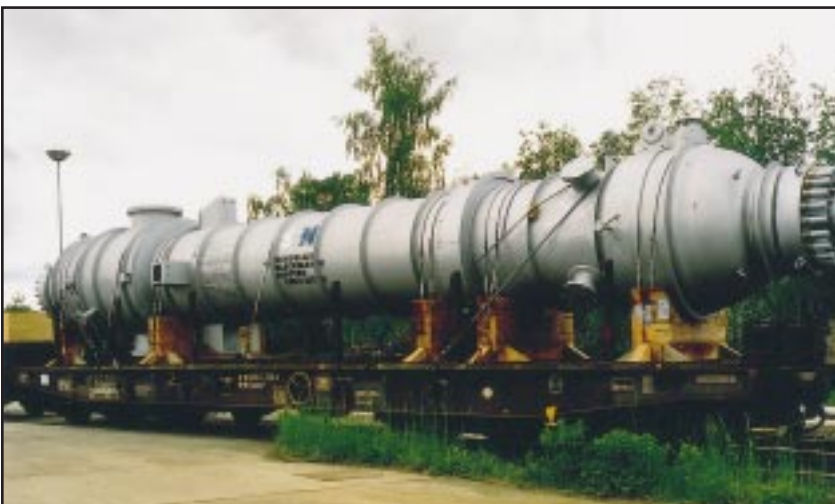
One of the first high pressure carbamate condensers made in Safurex. Courtesy: Schoeller-Bleckmann Nooter, Austria.
