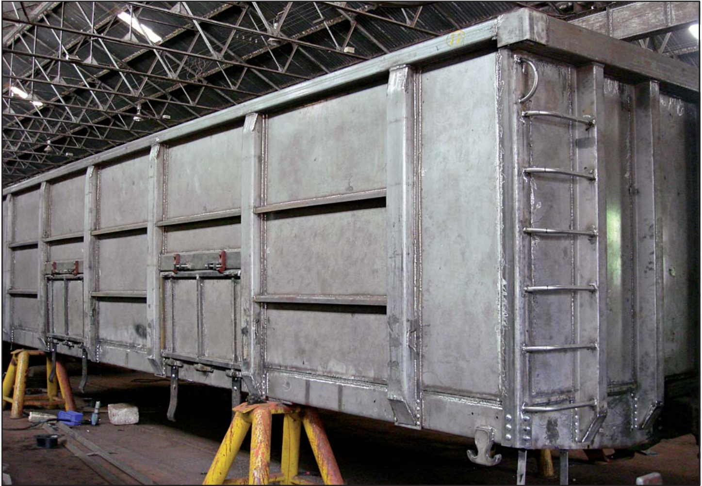
Unpainted sides of 409M wagon prototype
