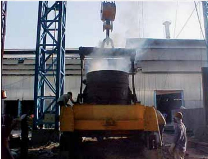
*Ladle transferring molten metal from AOD to continuous caster*
