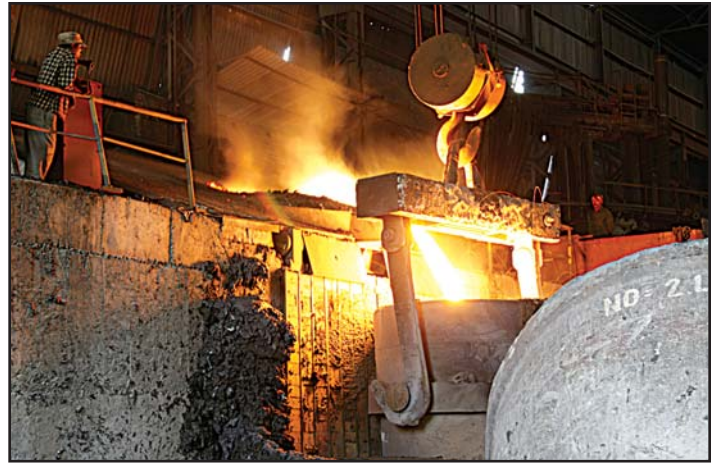
Liquid Stainless Steel is being transferred from induction furnace to AOD
