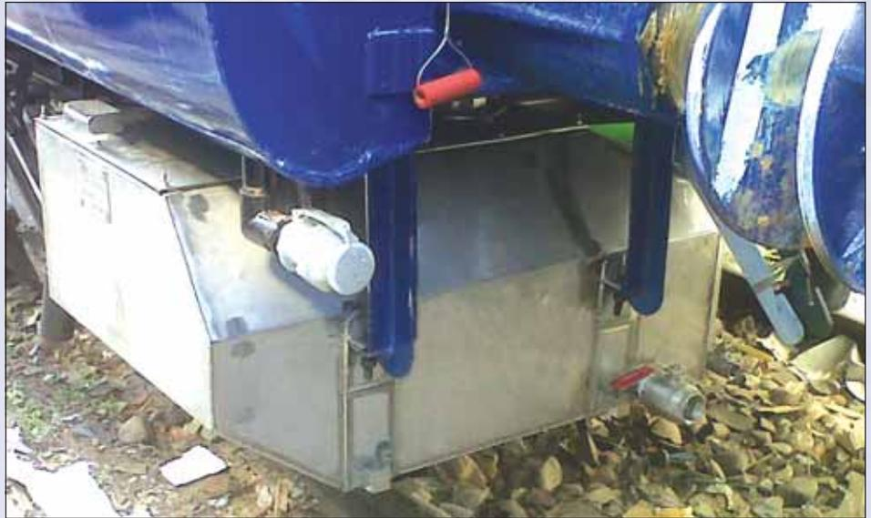
least eight long-distance trains. Now riding on the success from these trials, railway is planning to install 10,000 bio toilets based on the DRDO bio digester technology as proposed in 2012-13
