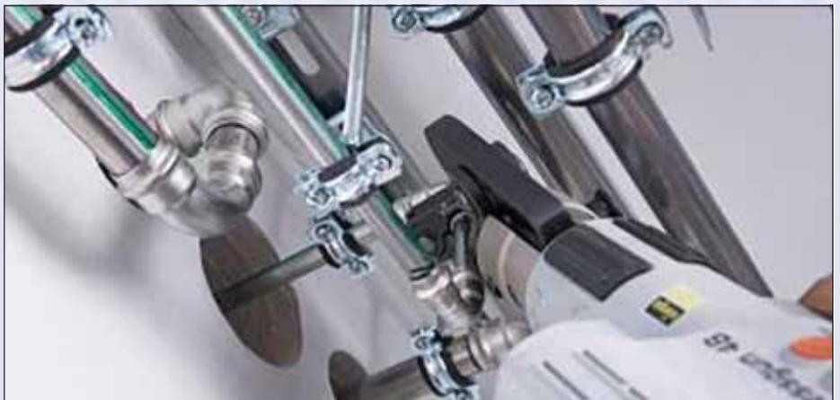
*The best tool for the Antarctic: Problem-free pressing of pipes at ambient temperatures around freezing and in the tightest of spaces – with the help of press rings. (Photo: Viega)*
