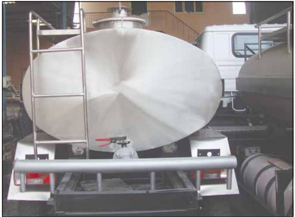
Fabricated SS water tanker with ladder and mud-guard all in SS 304
