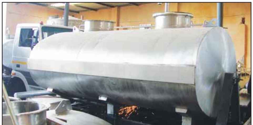
Stainless Steel 304 water tankers being mounted on chassis of the vehicle
