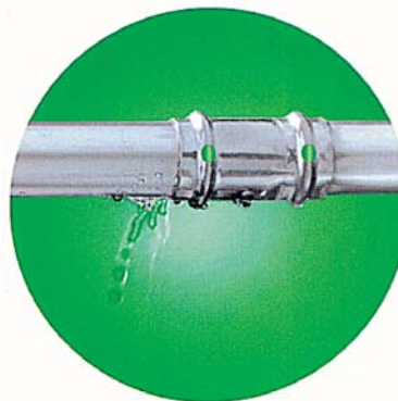
Sanpress Inox with SC-Contur: connections which have not been press-fitted = visible leakage during filling of the system.
