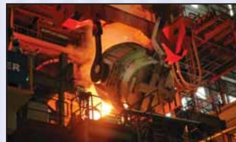
**Charging Liquid Steel into AOD Converter**
