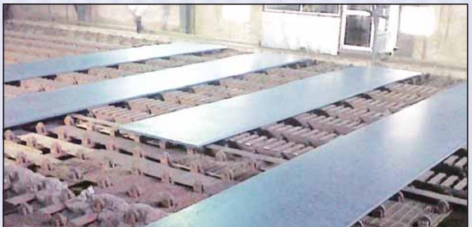
**Stainless steel plates at the cooling bed after rolling, annealing, quenching and hot levelling**
