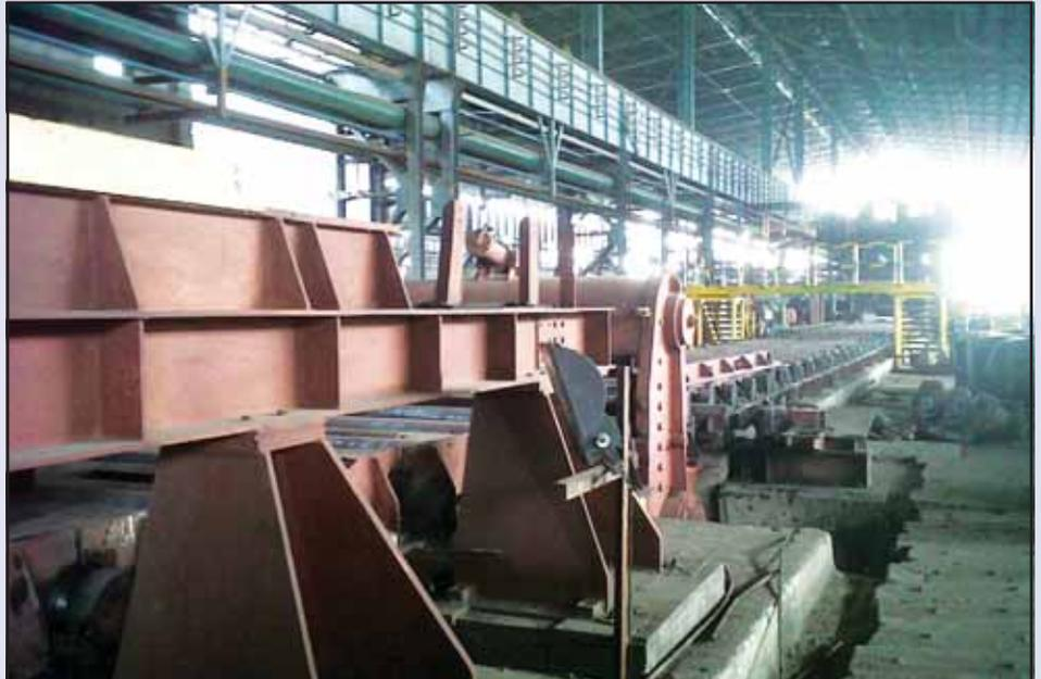
**BRG Plate Mill in operation for plate thickness 8mm & above, Widths 1250 – 2050mm**
