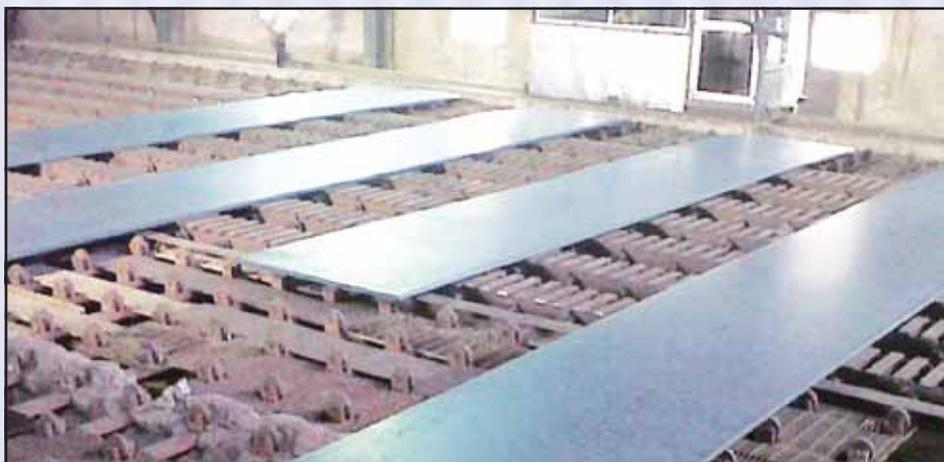
**Stainless steel plates at the cooling bed after rolling, annealing, quenching and hot levelling**
