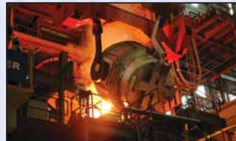
**Charging Liquid Steel into AOD Converter**
