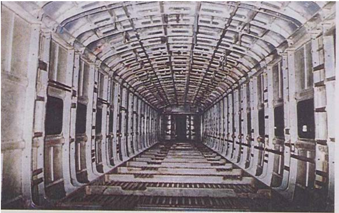
Stainless steel structural members (Photo courtesy ICF)
