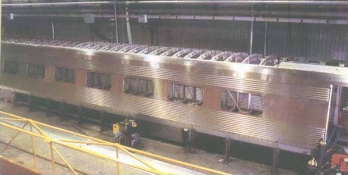
Future Perfect (A Swedish stainless rail coach under fabrication)
