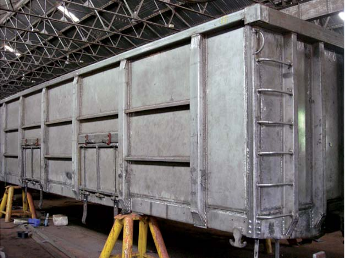
Unpainted sides of 409M prototype wagon
