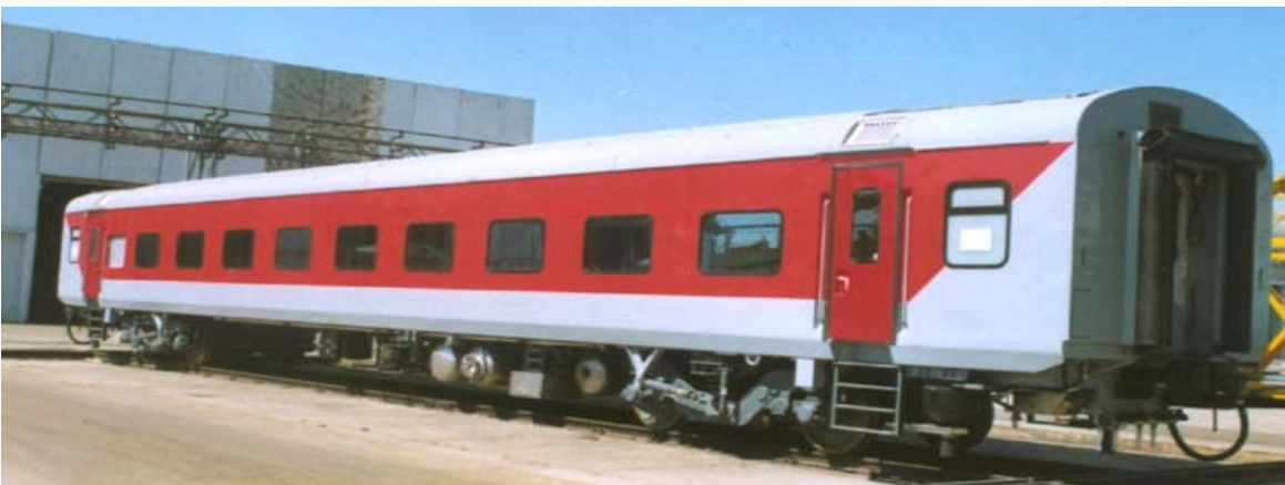
Delhi-Mumbai Rajdhani Express Painted 409M Stainless Steel coaches fabricated with LBH Design (Germany) at the Rail Coach Factory, Kapurthala.
