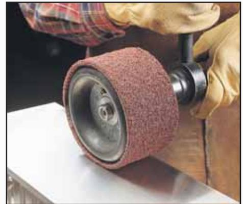
Different combinations of above products helps achieve different hairline or matt finishes and even helps restore the finish post the fabrication process. The process of finish generation includes 4 simple steps – weld grinding, blending, setting the grain, and final finishing. Using the above process sequence and choosing the right abrasive and tool helps achieve the desired finish.
