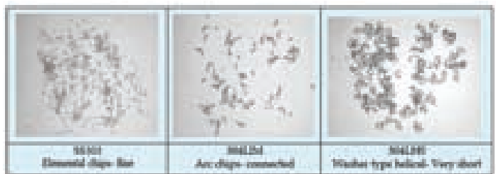
Figure 6. Chips from 304 LIM showed arc type chips compared to helical type for 304LHS.
