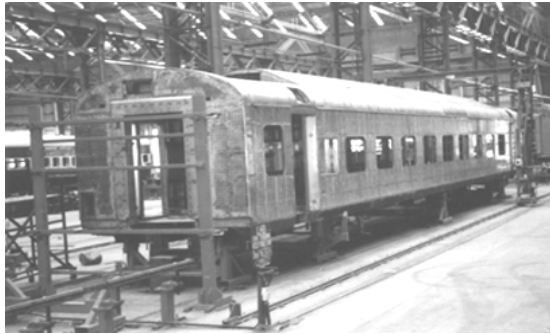
Left: A LHB stainless steel coach shell; Right: A prototype showing the interiors of a suburban train in Mumbai.
