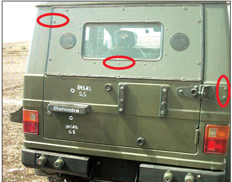
Some of the stainless steel 304 fasteners encircled.
