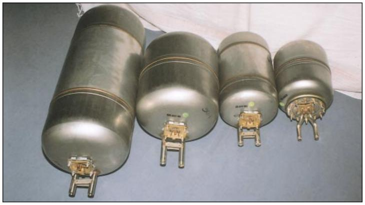
'Racold' brand water geysers (bottom left) and its stainless steel inner tanks (above) made by Merloni TermoSanitari (I) Ltd, Pune.
