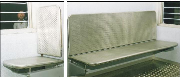
A close-up of the seats made of perforated stainless steel sheets.
