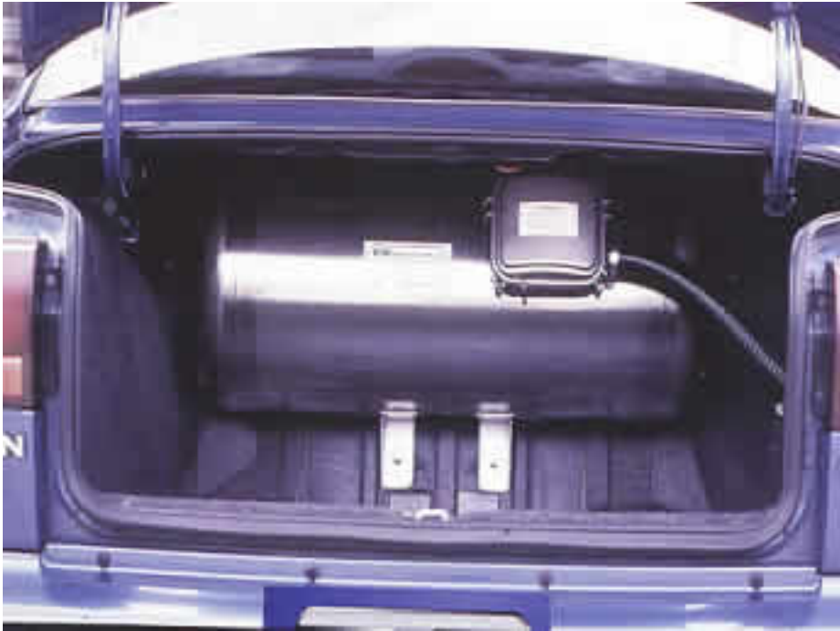
SS Auto LPG Tanks
