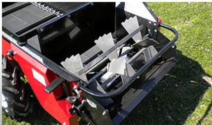
Martensitic stainless steel beater bars in a manure spreader
