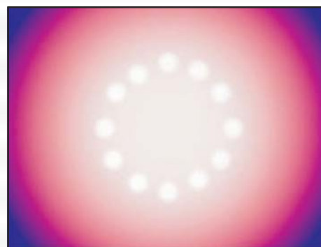
The white spots show the hottest regions where LPG flames directly hit the bottom of the stainless steel utensil; Red area shows moderate heat and blue areas are quite cold in comparison
