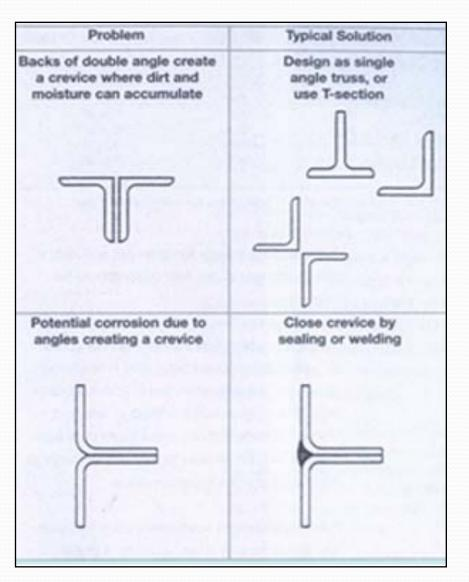
Seal joints or make wide enough to drain freely and avoid crevice corrosion.
